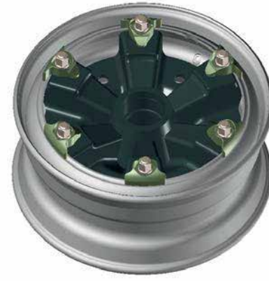
DEMOUNTABLE WHEELS, 15° DROP CENTRE FOR TUBELESS TYRES
